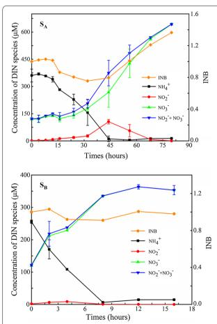
**Fig. 3** Time series for the concentrations of ammonium, nitrite and nitrate in the activated sludge of the aeration tank in Xinfeng WWTPs. Error bars represent standard variation (SD, n = 3)
