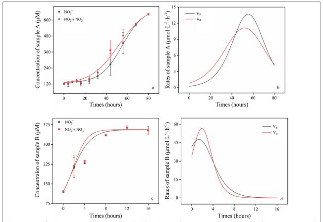
Fig. 1 Boltzmann fitted curves (**a**, **c**) and differential curves (**b**, **d**) from Boltzmann fitting equations of the DIN time series for instantaneous rates of ammonia oxidation (Va) and nitrite oxidation (Vn) of the water samples
