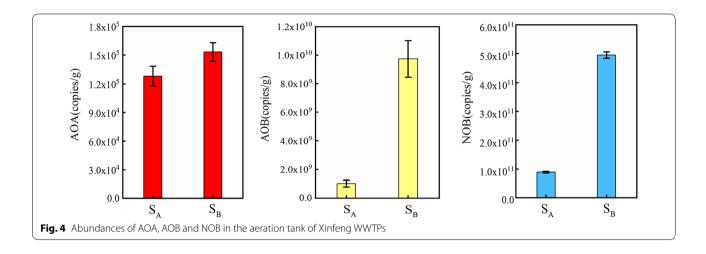
qPCR method. The abundance of AOA was the lowest in the microbial communities, ranging from  $1.2 \times 10^5$  to  $1.5 \times 10^5$  copies/g sludge (Fig. 4). In comparison, the abundance of AOB was 4 orders of magnitude higher than AOA, ranging from  $1.0 \times 10^9 - 9.7 \times 10^9$  copies/g sludge. However, the abundance of NOB *Nitrospira* was found to be 1-2 orders of magnitude higher than that of AOB.
