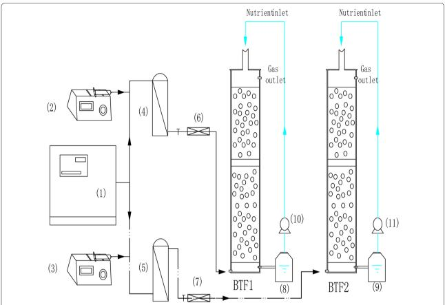
Fig. 1 The schematic of BTFs. (1) Air compressor, (2) (3) syringe pump, (4) (5) mixing chamber, (6) (7) three-way valve, (8) (9) nutrient-holding tank, (10) (11) peristaltic pump
