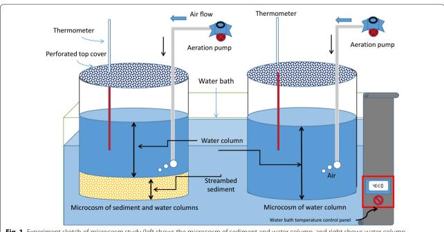
**Fig. 1** Experiment sketch of microcosm study (left shows the microcosm of sediment and water column, and right shows water column microcosm)
