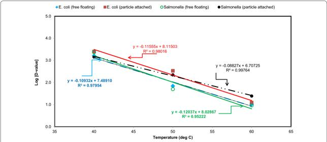
Fig. 9 Relationships between temperature and thermal reduction time (D-value) for Salmonella and E. coli O157:H7. The D-values were estimated from Table 1 [D-value = -1/(slope)]
