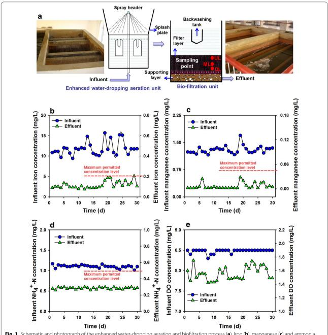
Fig. 1 Schematic and photograph of the enhanced water-dropping aeration and biofiltration process (a). Iron (b), manganese (c) and ammonia (d) removal effects and the DO variation (e) in the enhanced system
