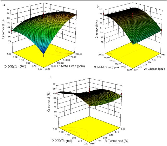
Fig. 3 Three dimensional plots of *A. niveus*. **a** Three-dimensional plot of residual Cr(VI) as a function of metal dose and glucose at constant tannic acid (2.75%) and  $NH_4CI$  (1 g/L). **b** Three-dimensional plot of residual Cr(VI) as a function of metal dose and tannic acid at constant glucose (0.5 g/L) and  $NH_4CI$  (1 g/L). **c** Three-dimensional plot of residual Cr(VI) as a function of  $NH_4CI$  and metal dose at constant glucose (0.5 g/L) and tannic acid (2.75%)
