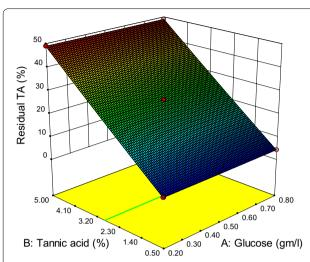
**Fig. 4** Three-dimensional plot of residual tannic acid as a function of tannic acid and glucose at constant  $NH_4CI$  (1.0 g/L) and metal dose (125 ppm)
