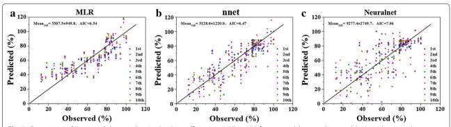
Fig. 7 Comparison of three models to predict zinc leaching efficiency. a MLR model; b nnet model; c neuralnet model. 50 random samples were used to construct the models, and then the remaining 30 samples were predicted (reshuffled 10 times)
