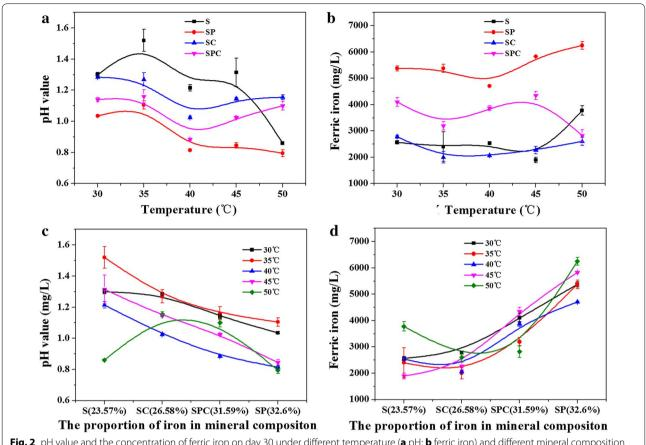
Fig. 2 pH value and the concentration of ferric iron on day 30 under different temperature (**a** pH; **b** ferric iron) and different mineral composition (**c** pH; **d** ferric iron)
