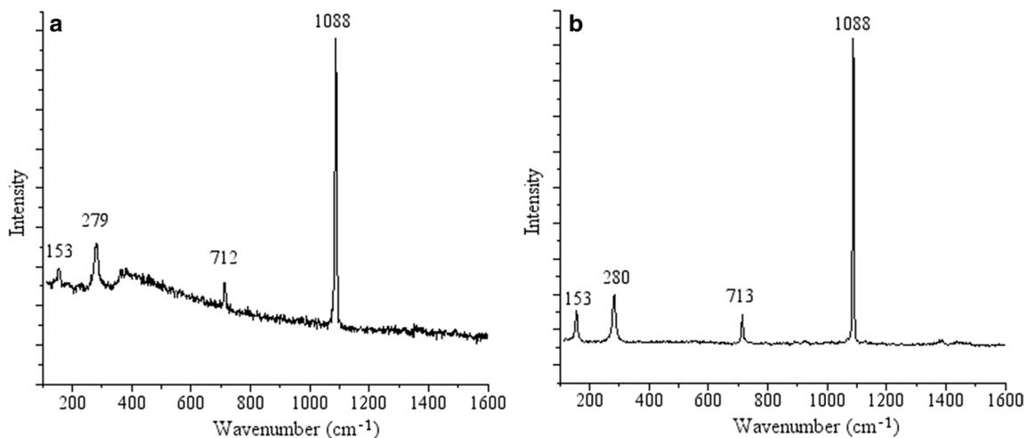
**Fig. 3** **a** Raman spectra of biomineralized calcium carbonate minerals in a *P. aeruginosa* biofilm. The highest Raman shift intensity appears at  $1088\text{ cm}^{-1}$ , indicating the presence of carbonate minerals. The primary peaks match those in a calcite standard spectrum (shown in **b**), indicating that the biomineralized deposits are calcite and not aragonite
