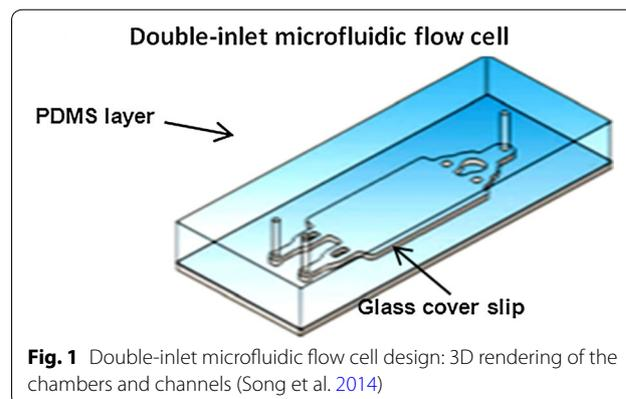
**Fig. 1** Double-inlet microfluidic flow cell design: 3D rendering of the chambers and channels (Song et al. 2014)
