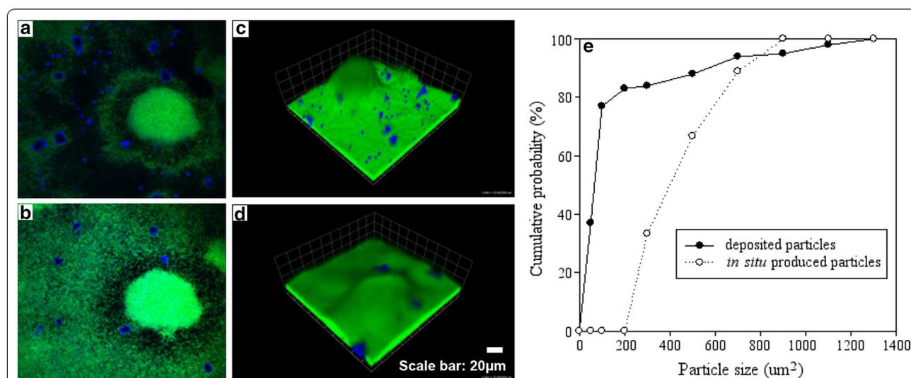
**Fig. 4** Biofilm traps precipitated fine calcite particles from bulk flow: **a–c** are under deposition mode and **d** is under suspension mode (control). **a** and **b** are xy planes of the same biofilm colony but at different depths. **a** is near bottom and **b** is near top. Mineral particle size distributions of **a** and **b** are plotted in **e**
