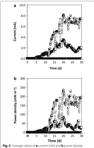
**Fig. 2** Average values of **a** current (mA) and **b** power density (mW m $^{-2}$ ) were analyzed throughout the operation period (pH 7.0: open circles, pH 5.5: open squares, and pH 4.0: open triangles)
