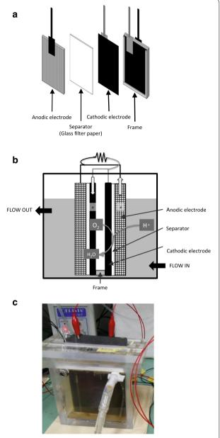
**Fig. 1 a** Schematic diagram of anode and air cathode electrodes, **b** microbial fuel cell (MFC) and **c** photograph of the MFC used in this study
