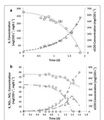
**Fig. 1** Typical batch and modeling (data fitting) results for **a**  $N_2O$  as sole electron acceptor, **b**  $NO_3^-$  as sole added electron acceptor; model sCOD (dotted line), model biomass (— =), model  $NO_3^-$  (— — -), experimental sCOD (square), experimental biomass (diamond), experimental  $NO_3^-$  (circle), experimental  $NO_2^-$  (triangle)
