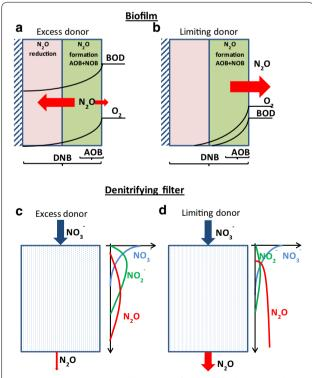
**Fig. 3** Top panels theoretical behavior of denitrifying bacteria in biofilms under (**a**) excess or (**b**) limiting electron donor conditions. *Lower panels* theoretical nitrogen profiles in a denitrifying filter in presence of (**c**) excess or (**d**) limiting electron donor
