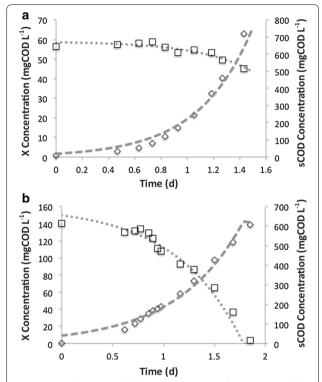
**Fig. 2** Typical batch tests for the determination of apparent rates for **a**  $NO_3^-$  and **b**  $NO_3^-$  plus  $N_2O$ . Model sCOD (dotted line), model biomass (dashed line), experimental sCOD (square), experimental biomass (diamond)
