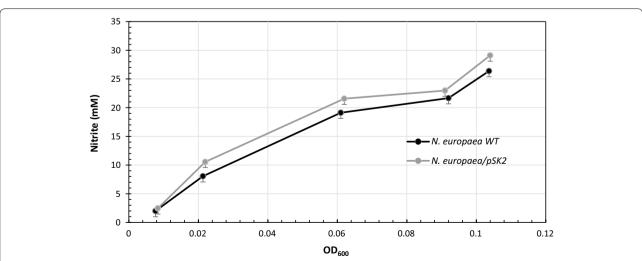
**Fig. 5** Ammonia to nitrite conversion as a function of cell mass (OD<sub>600 nm</sub>) for growing cultures of *N. europaea*[pSK2] and untransformed *N. europaea*. Each point is the average of 10 independent experiments; *europaea* indicate standard deviations.
