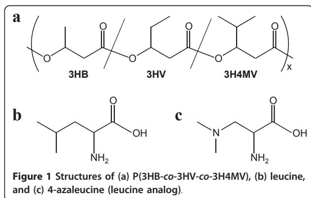
**Figure 1** Structures of (a) P(3HB-*co*-3HV-*co*-3H4MV), (b) leucine, and (c) 4-azaleucine (leucine analog).
