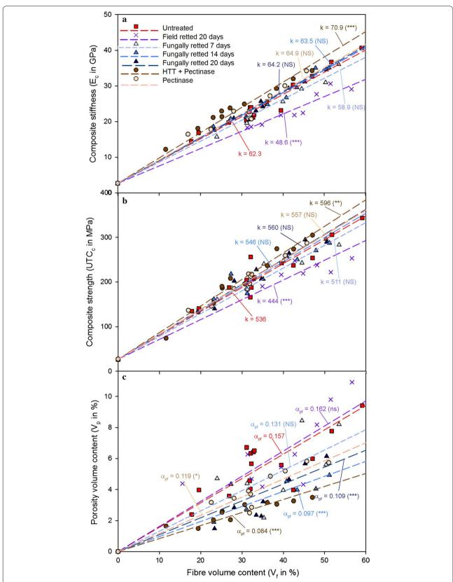
Fig. 4 Stiffness (a), UTS (b) and porosity (c) of composites reinforced with untreated and treated fibres versus fibre volume (V<sub>t</sub>) contents (k is slope of the linear regression model lines). Pectinase treatment was performed with and without prior autoclave treatment (HTT) at 1 bar (121 °C) for 30 min (Liu et al. 2016b)
