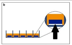
**Fig. 2** Sample preparation; ion irradiation of samples with missing irradiation of the sample's lower surfaces (**a**), placement of samples in well culture plates with paraffin wax (*arrow*) covering the sample's lower surface (**b**)
