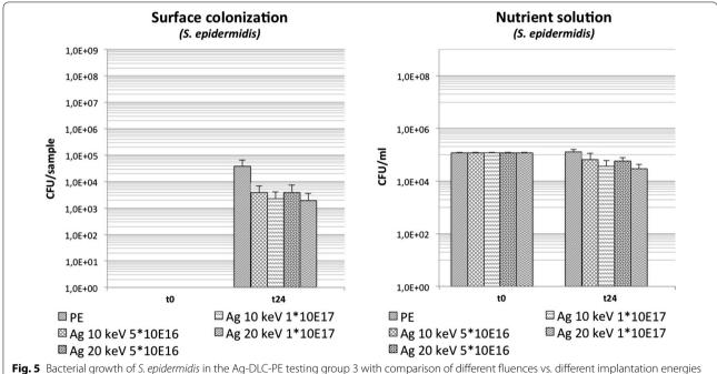
**Fig. 5** Bacterial growth of *S. epidermidis* in the Ag-DLC-PE testing group 3 with comparison of different fluences vs. different implantation energies (t = 0: before incubation; t = 24 h: after incubation)
