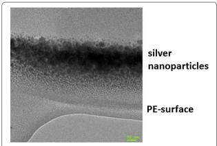
**Fig. 1** Transmission electron microscopy (TEM) image of silver nanoparticles of AG-DLC-PE; *notice* nanoparticles do not coat the PE surface but are embedded in the PE
